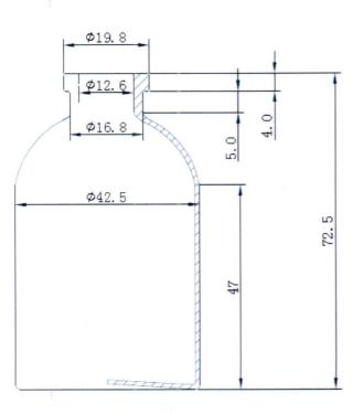
Filling Volume:54.0ml±1.5ml Height: 72.5mm±0.5mm Thickness of bottle-lip: 4.0mm±0.3mm Height of bottle-neck: 5.0mm±0.5mm Effective height of bottle-body: 47mm±1mm Outer diameter of bottle-mouth: 19.8mm±0.2mm Inner diameter of bottle-mouth: 12.6mm±0.2mm Outer diameter of bottle-neck: 16.8mm±0.3mm Body diameter: 42.5mm±0.4mm Material: Neutral borosilicate glass (PB-012) Sealing type: Chlorobutyl rubber stopper (PC-024) Cap: 20mm central hole cap (PA-041)
